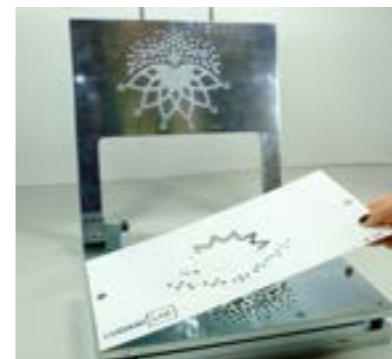
1 Put the first PVC mask onto the lower part of the mold.
