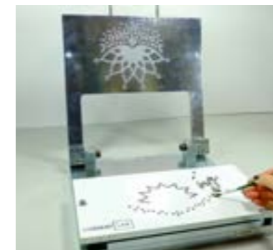
2 Sieve Rose Pins into the mask with the claws pointing upwards. Use one mask for each Rose Pin size and repeat the sieving step with all masks.
