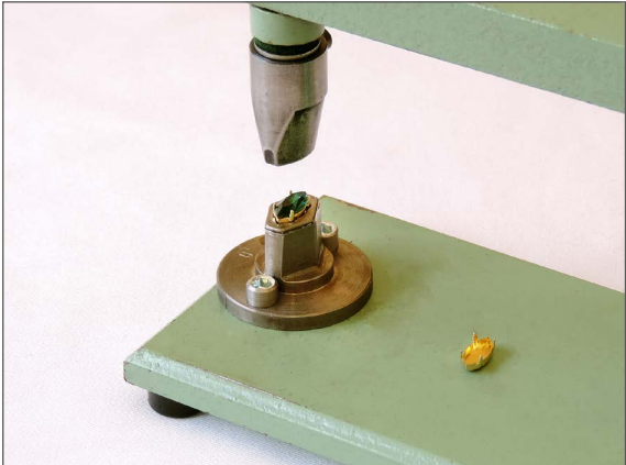
Simple device for setting bigger stones
