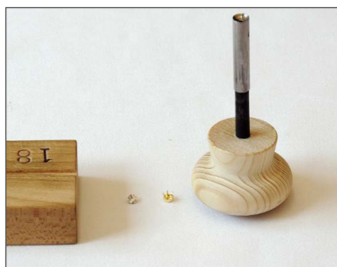
Setting and closing tool for individual cups
