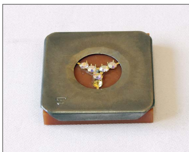
Device for manual setting of rhinestone balls
