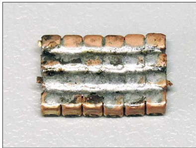
Optimal quantity of the solder
